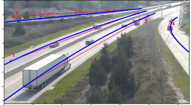
Figure 2. Parametric movement curves (blue) overlaid on camera scene and pre-defined movement curves and number (red). The green polygon is the region of interests and signals when a vehicle should be counted (upon exit). Movement 3 uses a first-order curve while movement 1,2, and 4 use second-order curves
